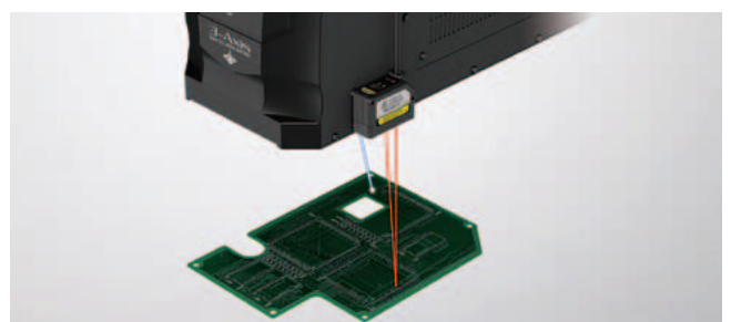
Control marking height
